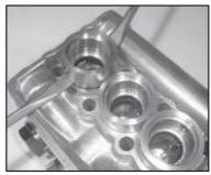
6) Remove seal adaptors (20) and weep return rings (25) from the valve casing.
