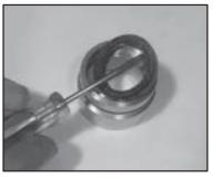
8) Remove the weep grooved seal (23 or 23B) together with pressure ring (24) out of the seal adaptor (20). Check O-rings (21).
